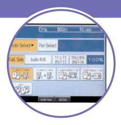
The Simplified Display shows only a select group of the most commonly used features, which makes it even easier for users to set up jobs.
